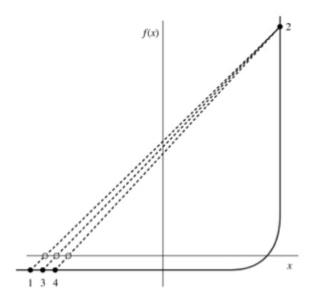
Better methods without derivatives such as Ridders or Brent's method combine these basic techniques: use these as default option and (optionally) switch to Newton once the solution is guaranteed for a higher convergence rate
