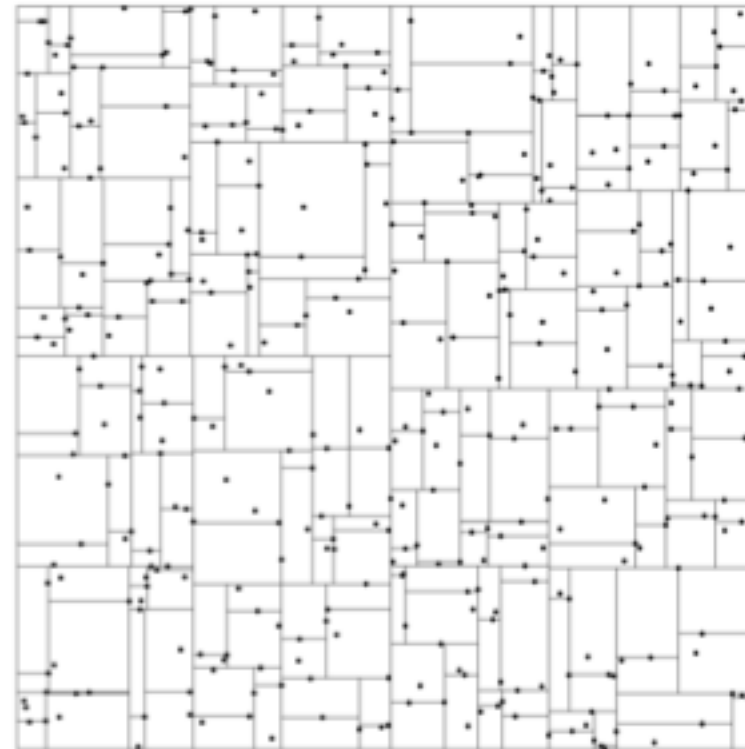
Figure 21.2.1. KD tree constructed from 1000 points in the plane. The first subdivision is visible as a full-height vertical line about halfway across the figure. The next subdivisions are horizontal lines, extending halfway across the figure. The subdivisions alternate between horizontal and vertical, and partition into (nearly) equal numbers of points at each stage. This tree terminates when there are either one or two points in a box (one of which is usually on the box boundary).
