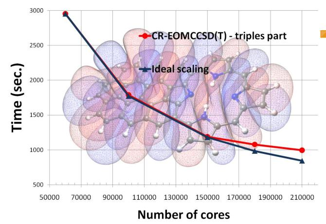
Scalability of the triples part of the CR-EOMCCSD(T) approach for the FBP-f-coronene system in the AVTZ basis set. Timings were determined from calculations on the Jaguar Cray XT5 computer system at NCCS.
