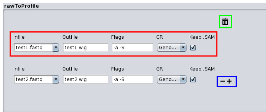
Figure A.10: A command component representing a raw-to-profile-process. The component has rows for input parameters (red), buttons to add and remove input rows (blue), and a button to remove the entire component (green).
